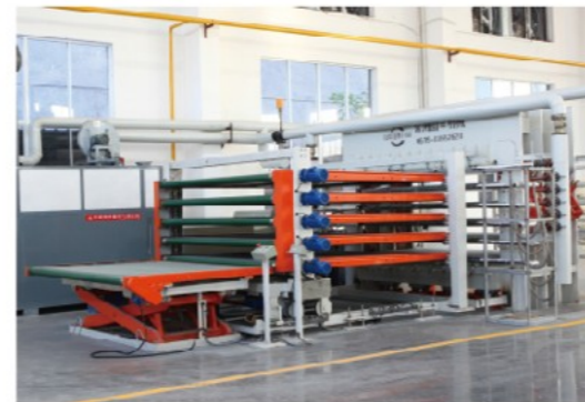
Capacity: 60–120 sheets/h Opening No: 5–10 layers
